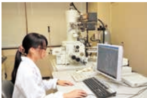
走査電子顕微鏡を用いた植物の微細構造観察 Observation of Ultra-fine structure of plant tissues using scanning electron microscope
