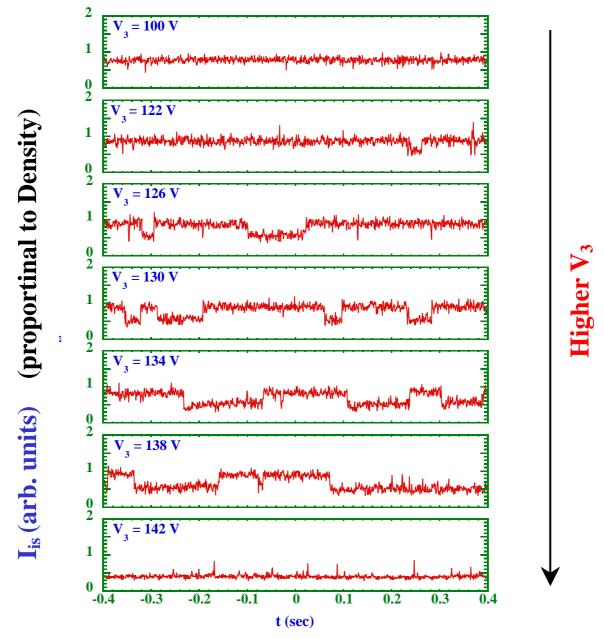
Time Evolution of Ion Saturation Current  $I_{is}$ , Changing Bias Voltage  $V_3$
