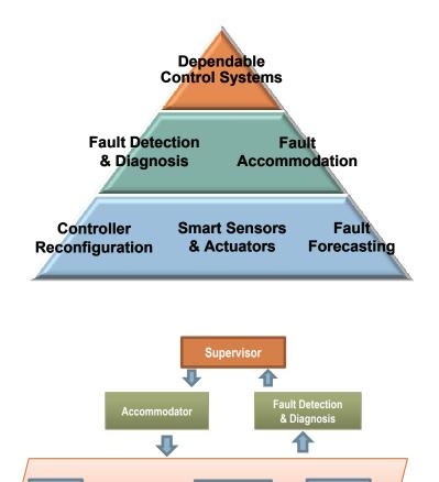
Typical architecture of an integrated dependable control system
