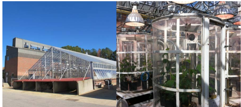
Figure 2. A greenhouse and an open-top chamber for studying the effect of O 3 on the biochemical responses of O 3 -tolerant and O 3 -sensitive soybeans
