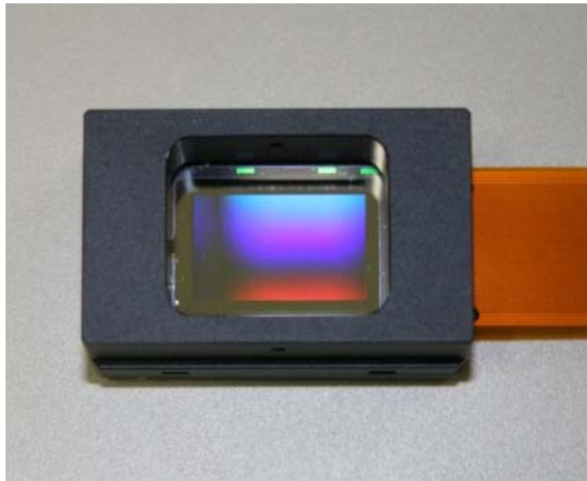
4k2k-SLM (JVC Kenwood) Resolution: 3,840 \times 2,400 Pixel pitch: 4.8 \mu\text{m} Central 3,200 \times 1,600 pixels were used.
