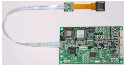
0.44" color LCD Resolution: ~QVGA (SONY LCX033AK)
