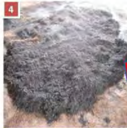
When the mound is totally carbonized, put water to stop charring.
