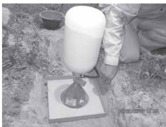
Figure 2: soil density test
