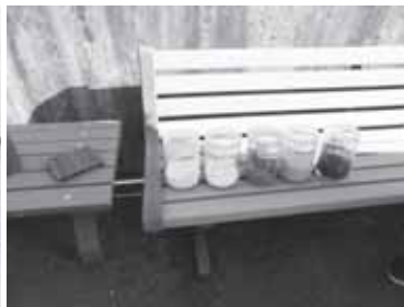
Fig.3 廃木材と廃プラから合成木材とベンチを作る/ Reproduce compound board and bench from waste wood and plastic
