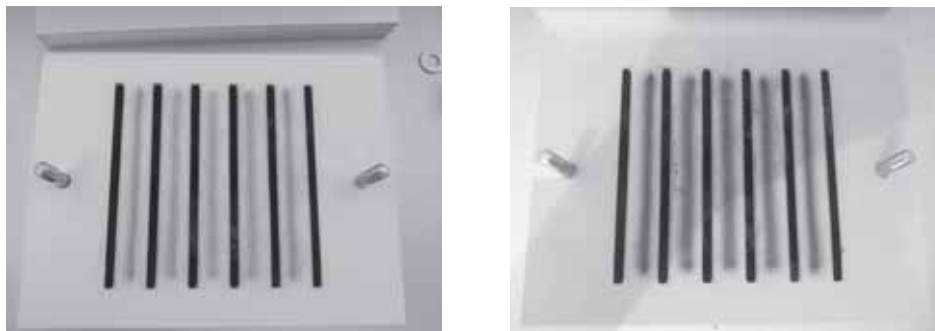
Fig. 6. Photograph of surfaces of filters used: (left) non-treated and (right) treated by palm oil
