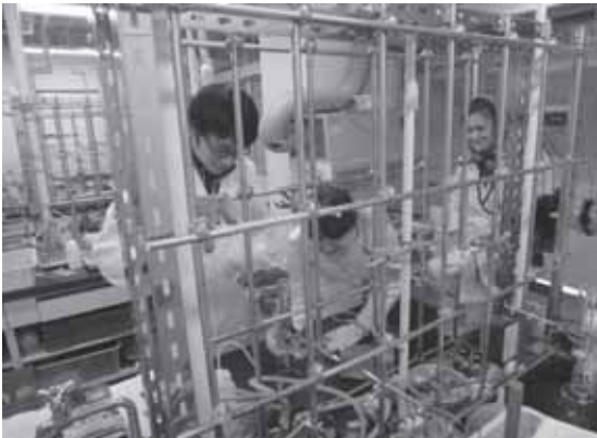
土壌による浸出水浄化試験/Soil evaluation test for the pollutant removal in the leachate
