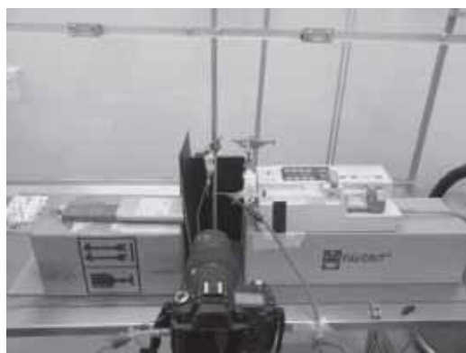
Fig. 5 System of particle generation
